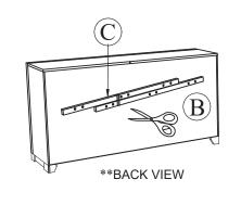
STEP 2: Turn the MIRROR SUPPORT RAIL (C) upward at the back of DRESSER (B), then Tighten with CSK SCREW (1). Place the MIRROR FRAME (A) on the top of DRESSER (B). Tighten with Flat Head Chipboard Screw (1).
