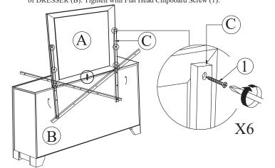
**STEP 3:** Tighten the Flat Head Chipboard Screw (2) as shown.
